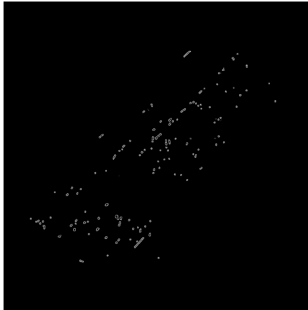
Figure 4.4: Defects detected with the use of Canny edge detector
