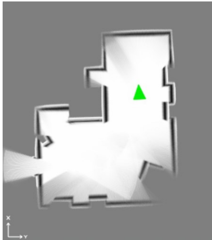
Figure 2.4: Laser-based map in simulation environment generated from CoreSLAM [5]
