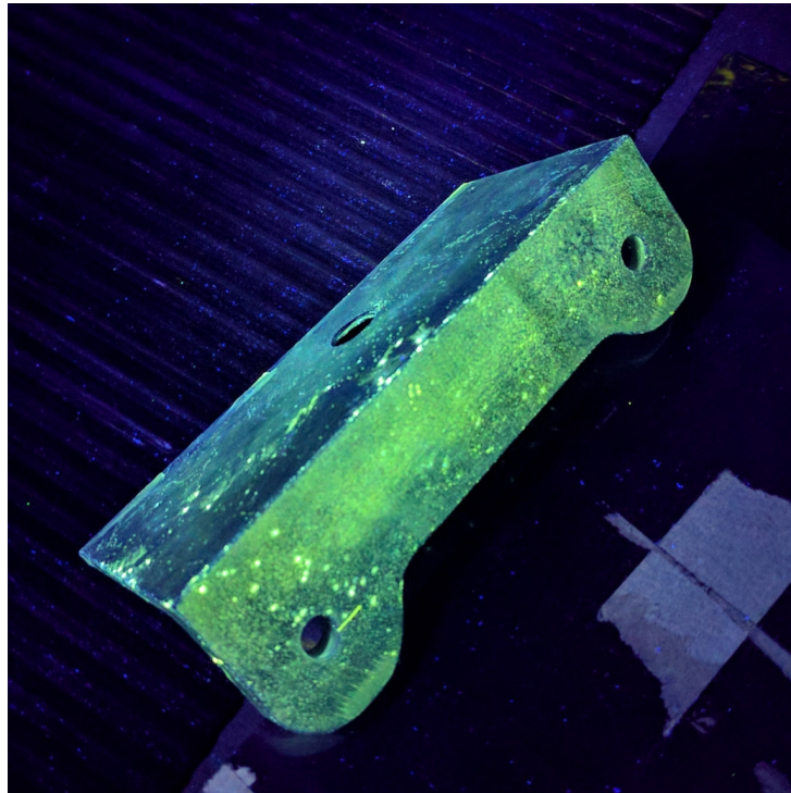
Figure 4.2: Sample after Penetrant Testing with numerous defects
